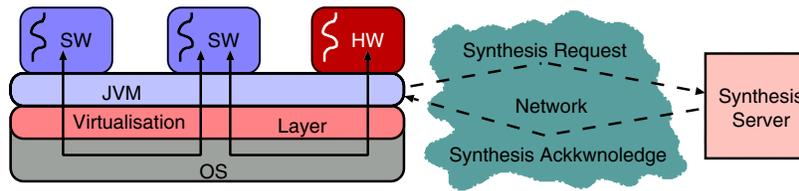
**Figure 7. Dynamic reconfiguration. JVM runs on top of the virtualisation layer. It requests migration of critical methods from software to hardware.**
