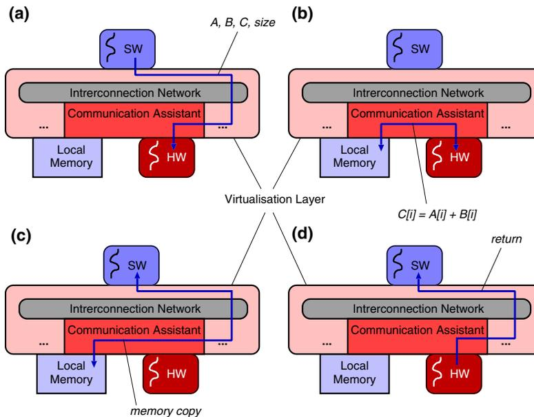
**Figure 5. Execution model. The software thread invokes a hardware thread through the virtualisation layer (a). The hardware thread accesses the local memory through the communication assistant (b). The virtualisation layer provides address translation and transparent memory copies (c). The hardware thread communicates the end of operation through the virtualisation layer (d).**
