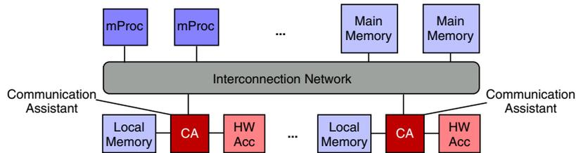
**Figure 4. Reconfigurable parallel architecture. Computing nodes (standard processors and hardware accelerators) communicate through a general interconnection network. Hardware accelerators are interfaced to local memories and to the rest of the system through standardised communication assistants.**
