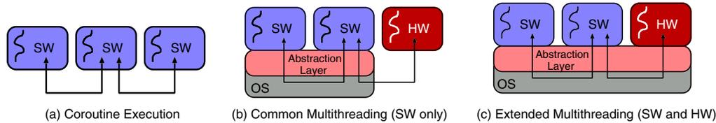
**Figure 1. Multithreaded programming model. Coroutine execution (a) is the first approach to multithreading without system-level support. Common multithreading (b) supported by an abstraction layer (i.e., standardised libraries and OS services) ignores the existence of hardware threads. Extended multithreading (c) supports seamless integration of hardware threads: programming is transparent and interfacing is portable.**
