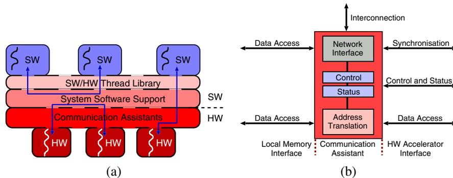
**Figure 6. Virtualisation layer and communication assistant: (a) software and hardware threads are hooked to the virtualisation layer; (b) the communication assistant defines interface signals and translates virtual addresses.**
