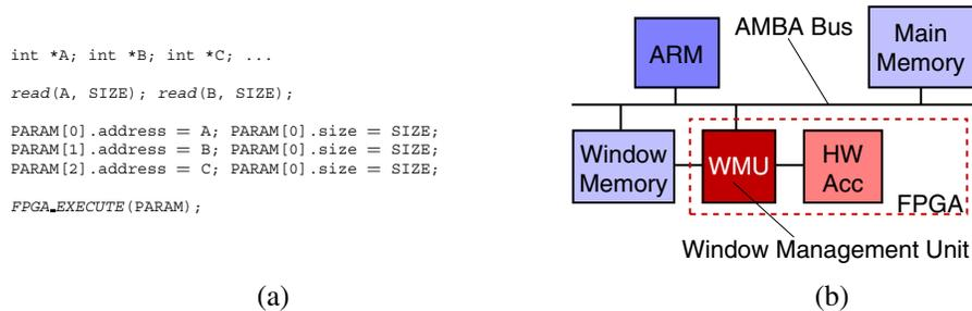
**Figure 8. Virtual memory window: (a) programming; virtual memory pointers are passed as-they-are to the hardware accelerator; (b) interfacing; the accelerator accesses local memory through the WMU.**
