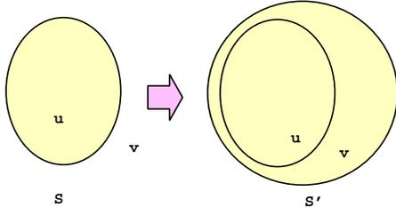
**Figure 6: Two nodes are related if any convex subgraph containing one of them can be extended to a convex subgraph containing both of them.**
