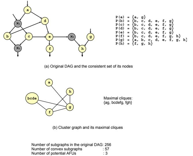
**Figure 9: An example of forming cluster graph from the original graph and enumerating its maximal cliques. The black nodes in the graph indicate forbidden nodes.**
