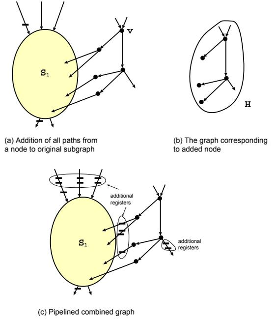
**Figure 5: Adding a single node and all paths from this node to the subgraph increases the speedup.**
