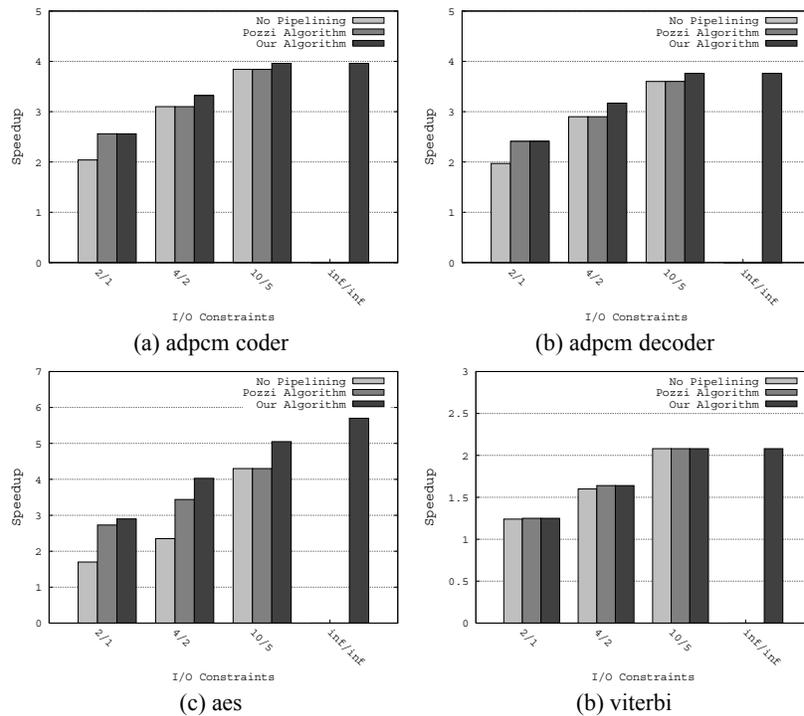
Figure 11: Comparison of the speedup values of AFUs generated by our algorithm with the state of art techniques.
