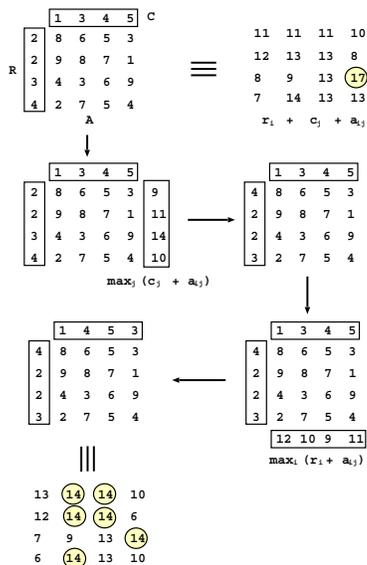
**Figure 10: Execution of ping-pong algorithm on a simple example. Note that in this case ping-pong finds the optimal solution only in two iterations.**
