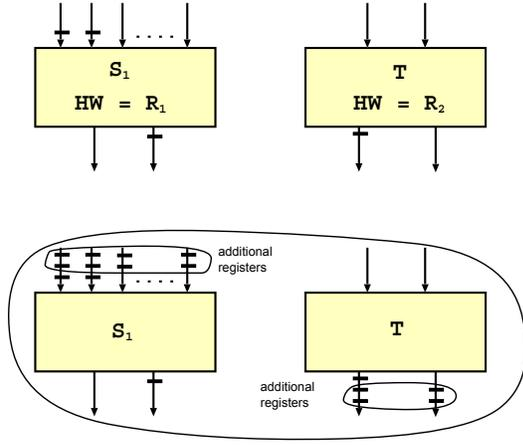
**Figure 4: Disjoint union of two convex subgraphs increases the speedup.**
