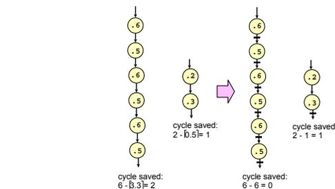
**Figure 2: An example showing that the relative merit of AFUs might change after pipelining Assume that software latency of each node is 1.0.**
