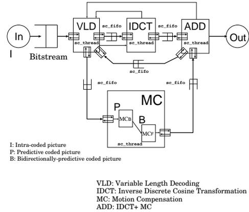
Figure 2. MPEG2 Video Decoder Data- and Control-Flow
