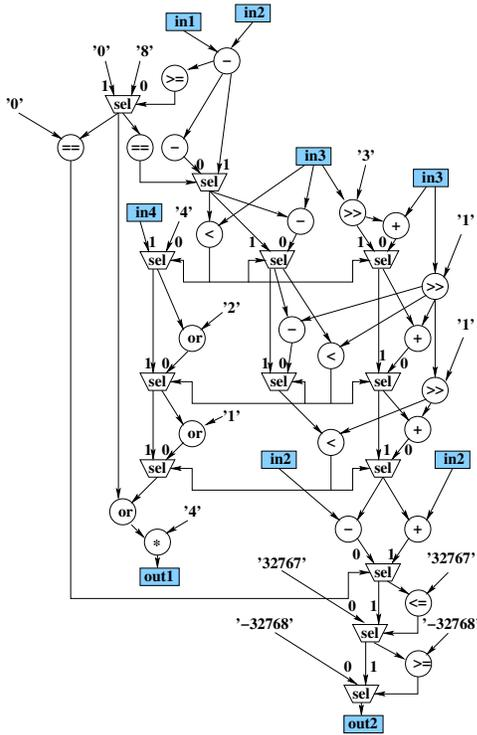
Figure 8: An ISE for ADPCM ENCODER (*adpcm-e*) having 4 inputs and 2 outputs; each operation node maps to a hardware component.
