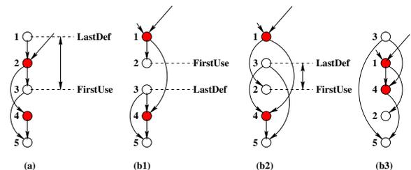
Figure 4: The ISE here is composed of the shaded instruction nodes. (a) An example showing the *LastDef* point and the *FirstUse* point; (b1) an example where it is not possible to insert the ISE under consideration; (b2) After code restructuring; (b3) positioning of the ISE between *LastDef* and *FirstUse*.
